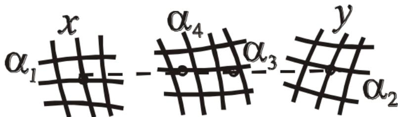
Figure: A nomographic construction of a relation between 6 variables
