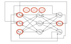
Directed graph representing the equivalent IC. Demand  $\mathbf{d}=(1,3,2);$  set not containing a cycle is  $(F_{1,\oslash},F_{1,2},F_{1,3},F_{1,23},F_{3,\oslash},F_{3,2},F_{2,\oslash}).$
