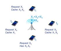
Example of a IC. If the TX serves the requested messages one by one, 4 transmissions are necessary. If instead it uses coded transmission, 2 transmissions suffice. 50% bandwidth savings!
