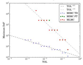
Maximum number of degrees of freedom of a sample PDE solve for different TOL values. This is an indication of required memory.
