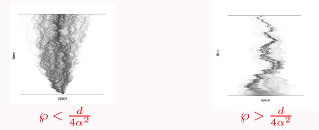
Explosive separation of trajectories versus implosive collapse (from Falkovich-G.-Vergassola Rev. Mod. Phys. 73 (2001))
