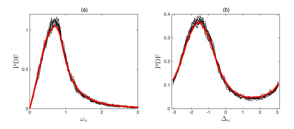
PDFs at stochastic constant state of the traveling wave (n = 15,...,25) vs. PDFs of turbulent dynamics in inertial interval for the statistical equilibrium
