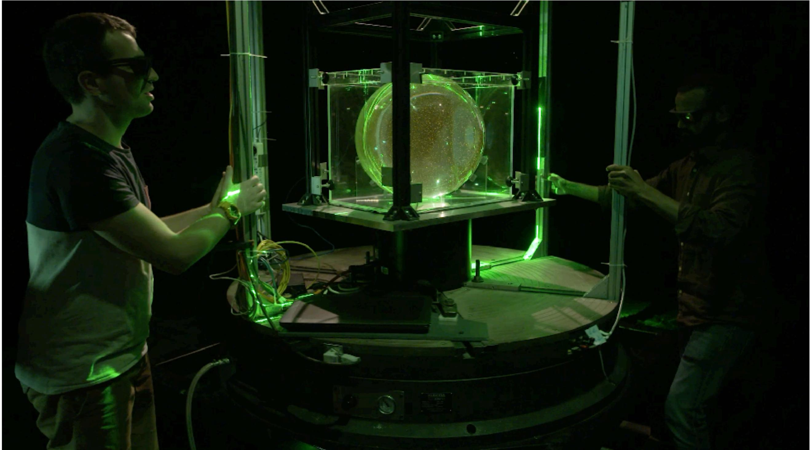
size  $\sim 50\text{cm}$ , rotation up to  $90\text{rpm}$   $\rightarrow E=5 \times 10^{-6}$
