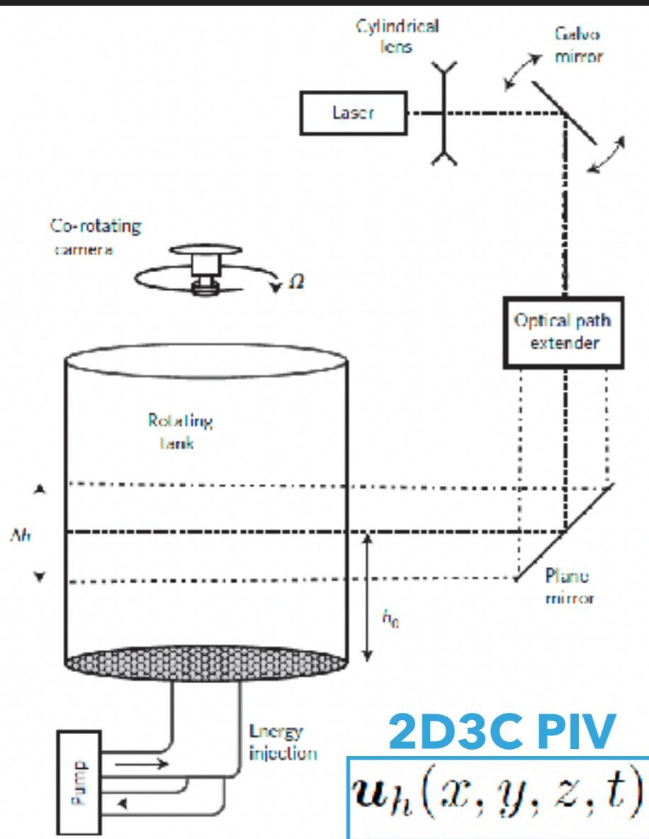
**Figure 1 | Experimental set-up.** A laser sheet illuminates a rotating Plexiglas cylinder filled with water and seeded with tracer particles. Using a galvo mirror, the sheet is repeatedly swept vertically through 30 horizontal planes, in the range  $\Delta h = 25.6$  cm around height  $h_0$ . A co-rotating camera ( $\sim 750$  frames per second) images the light scattered from the tracer particles.
