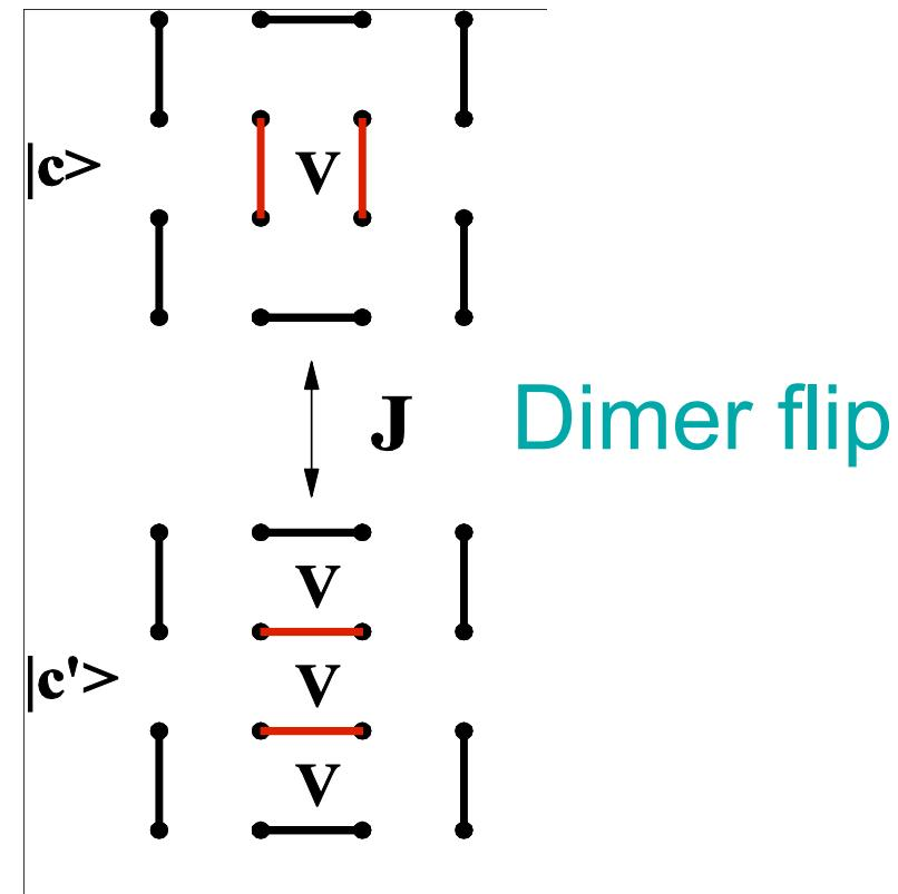
$$H_{\text{QDM}} = \sum_c e_c |c\rangle\langle c| - J \sum_{c,c'} |c\rangle\langle c'|$$
