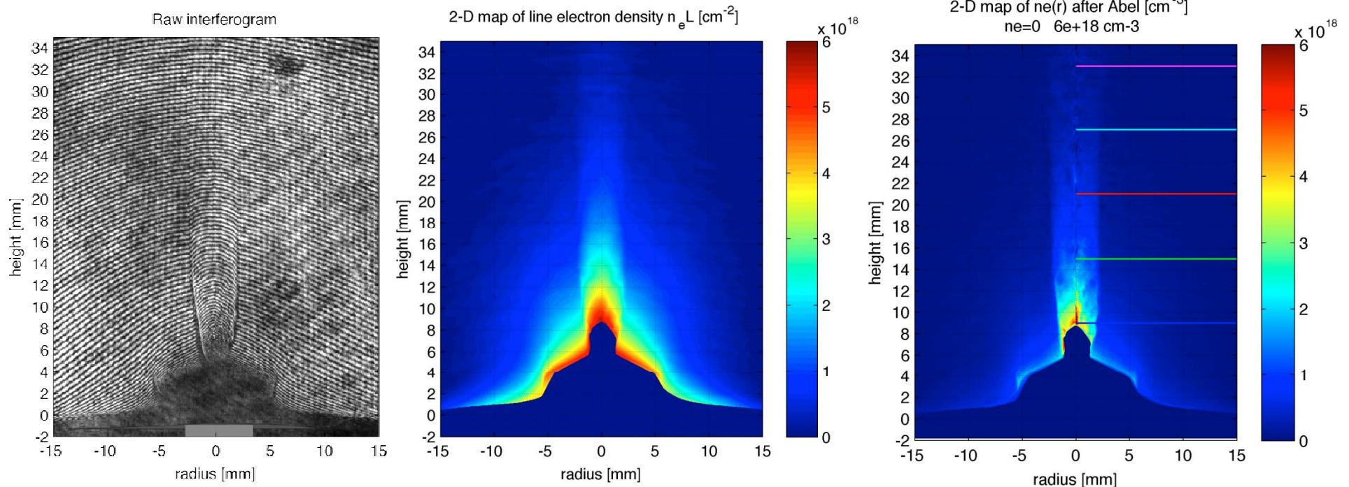
**Shape / collimation of the jet are similar to observed in XUV emission**
