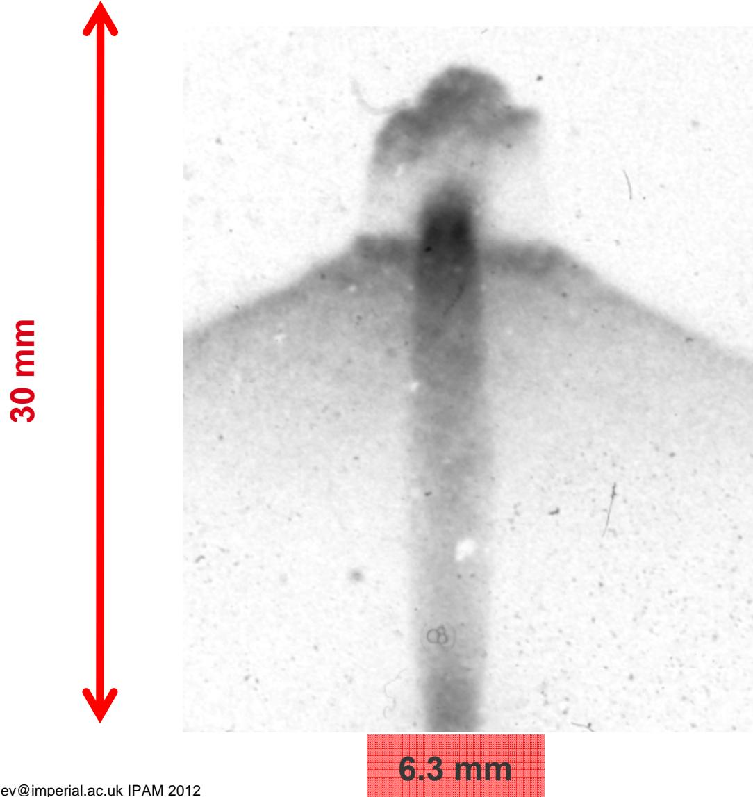
Presence of argon does not disrupt formation of a collimated jet
