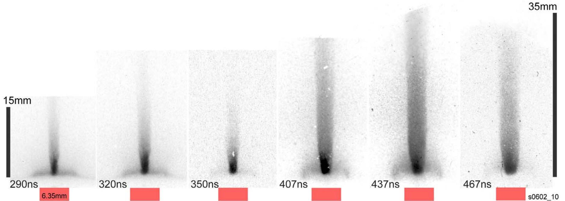
**Highly collimated jet , plasma is flow supported for ~350ns**
