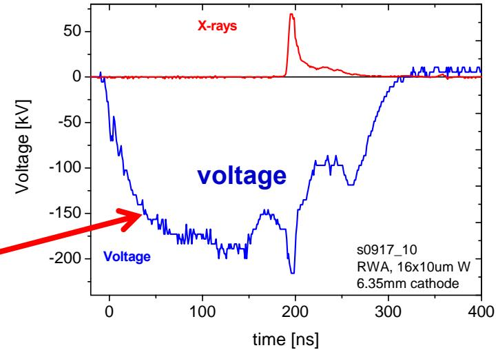
High voltage at the base of the jet at the time of the jet formation
