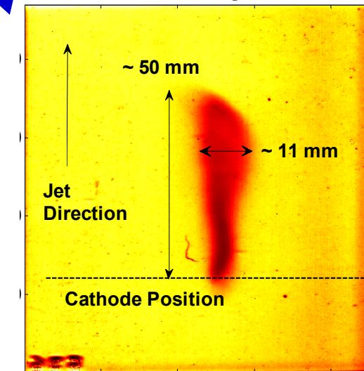
Presence of proton trapped in the magnetic cavity
