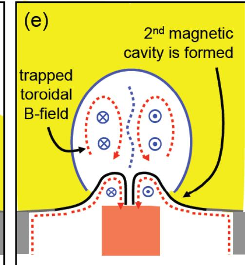
Plasma expanding from the electrodes close the gap and reconnects the current
