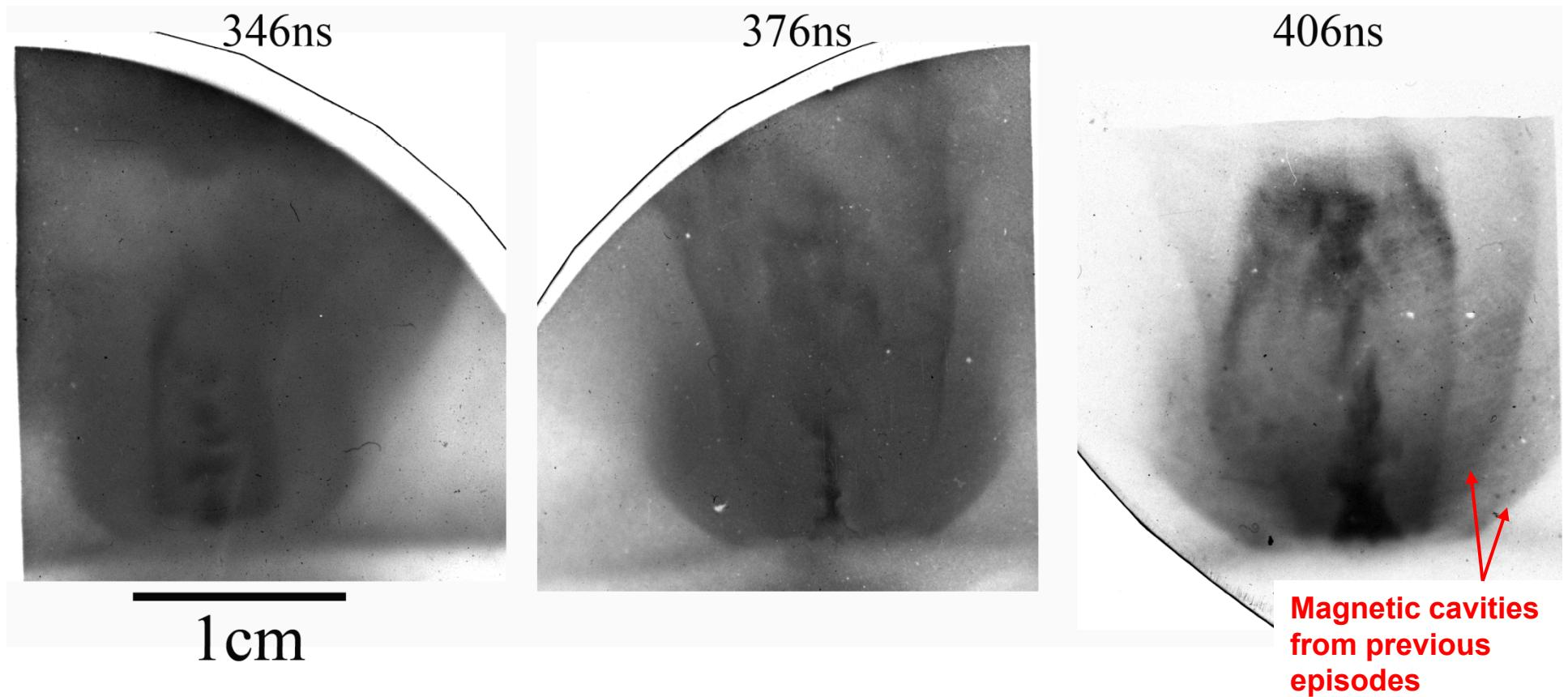
Reduced radial expansion of the subsequent magnetic cavities
