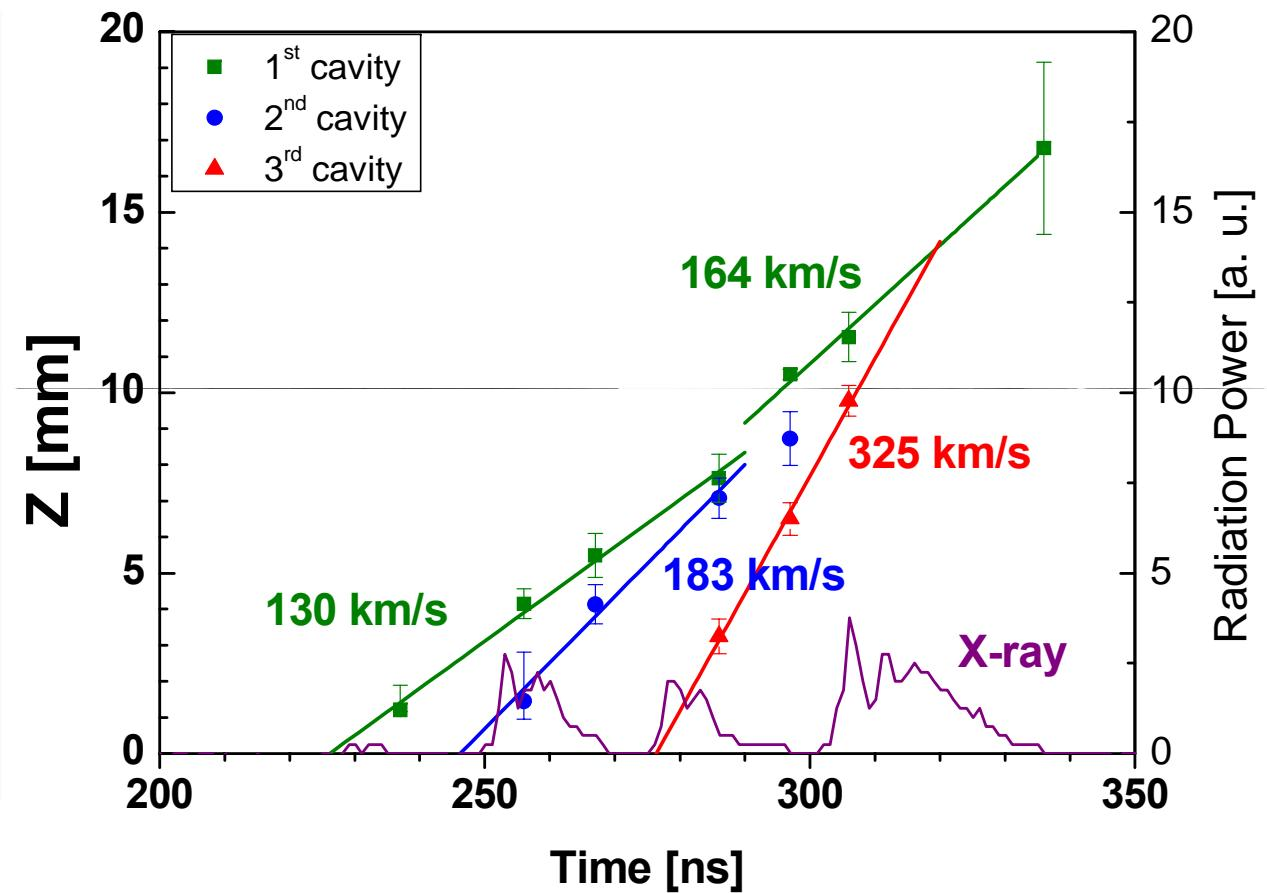
Subsequent magnetic cavities move faster
