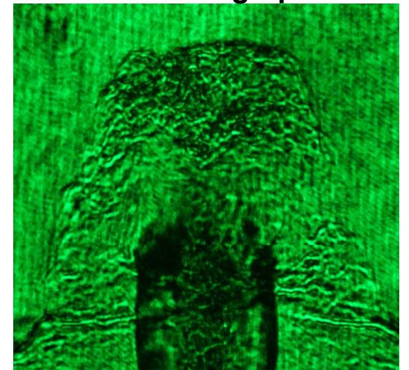
High compression in the shock due to radiative cooling
