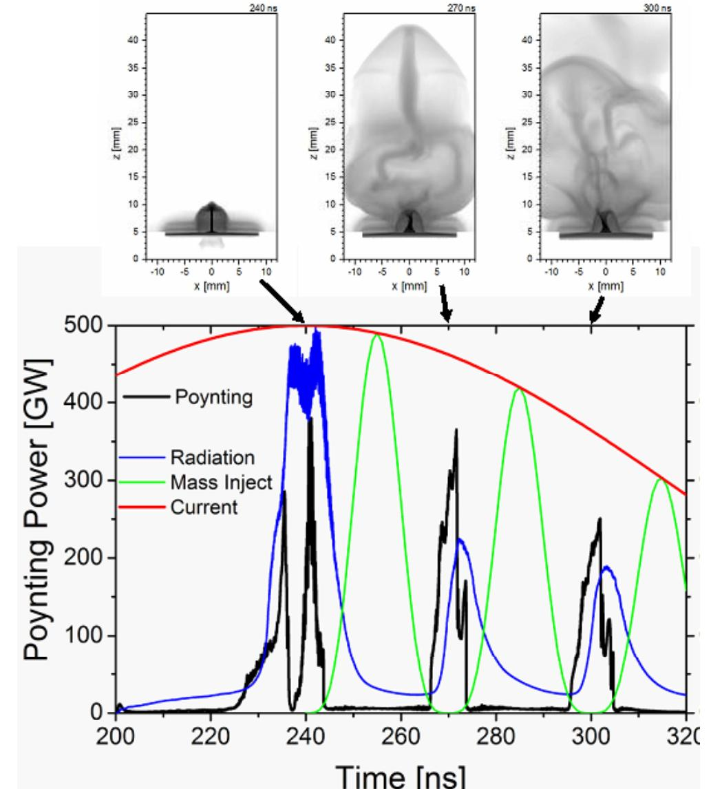
The reconnection of current is not simulated, instead mass is injected into the gap with  $dm/dt$ , proportional to the radiation power from the jet
