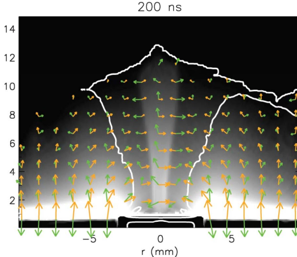
Toroidal magnetic field ( $B_\phi$ ) diffuses through the foil
