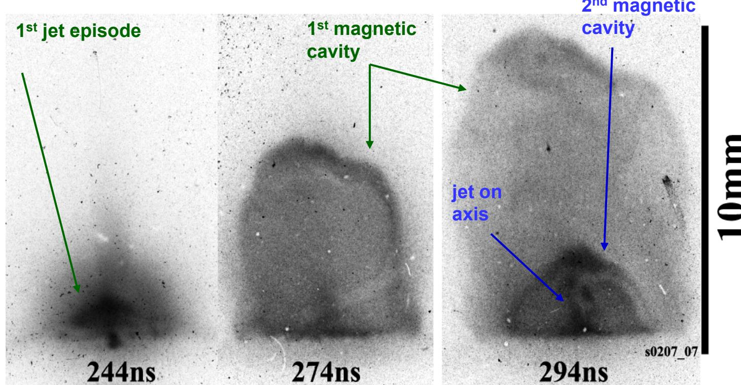
Reconnection of current at the base produces several magnetically driven bubbles
