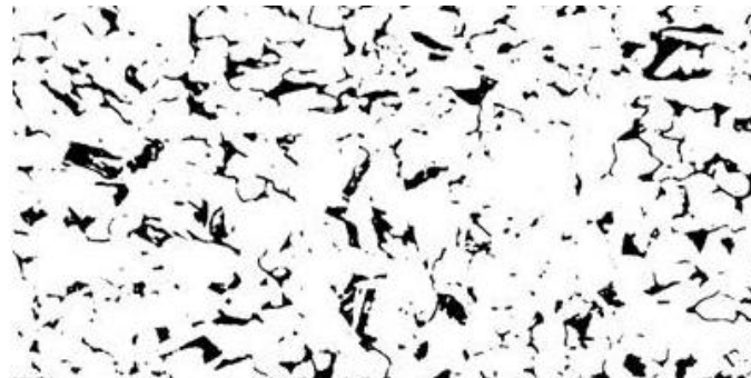
fully annealed at 920 °C
