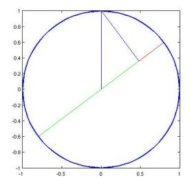
The loss is the length of the red line segment; the range is the combined lengths of the red and green line segments.
