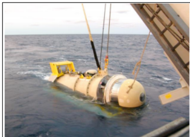
Figure 1: BP's Wolfspär ® prototype low-frequency seismic source being retrieved during operational testing at the Gulf of Mexico systems integration test in 2014.
