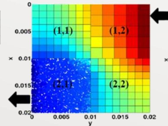
Mortars are finite element based function spaces forming the interface conditions between subdomains.
