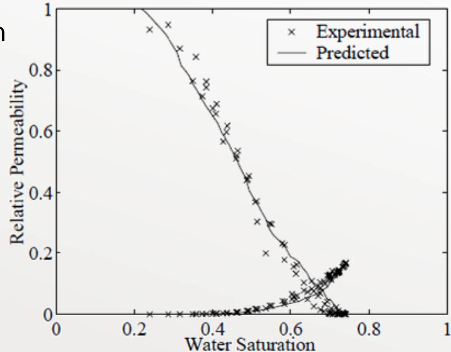
Figure 8: Predicted waterflooding relative permeability for water-wet Berea sandstone (lines) compared to experimental data by Oak (crosses)<sup>31</sup>.
