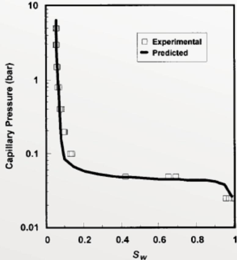
Fig. 13— Comparison between predicted and measured primary drainage capillary pressure for the water-wet Bentheimer sandstone.
