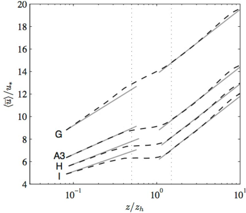
$$z_{0,hi} = z_h \left( 1 + \frac{D}{2z_h} \right)^\beta \exp \left\{ - \left[ \frac{\pi C_T}{8\kappa^2 s_x s_y} + \left( \ln \left[ \frac{z_h}{z_{0,ground}} \left( 1 - \frac{D}{2z_h} \right)^\beta \right] \right)^{-2} \right]^{1/2} \right\}$$
