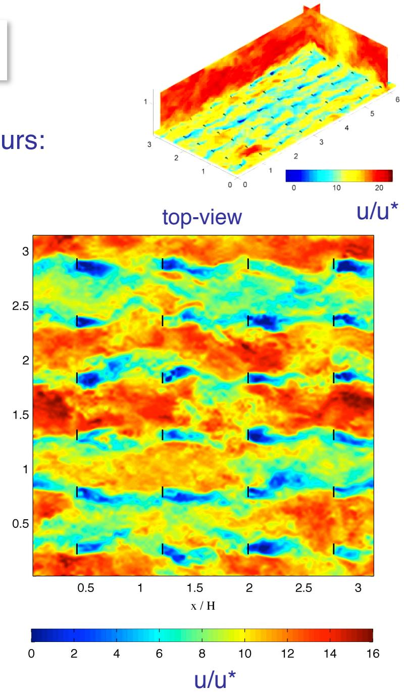
**In-silico wind farm (Large-Eddy-Simulation) JHU-LES code**
