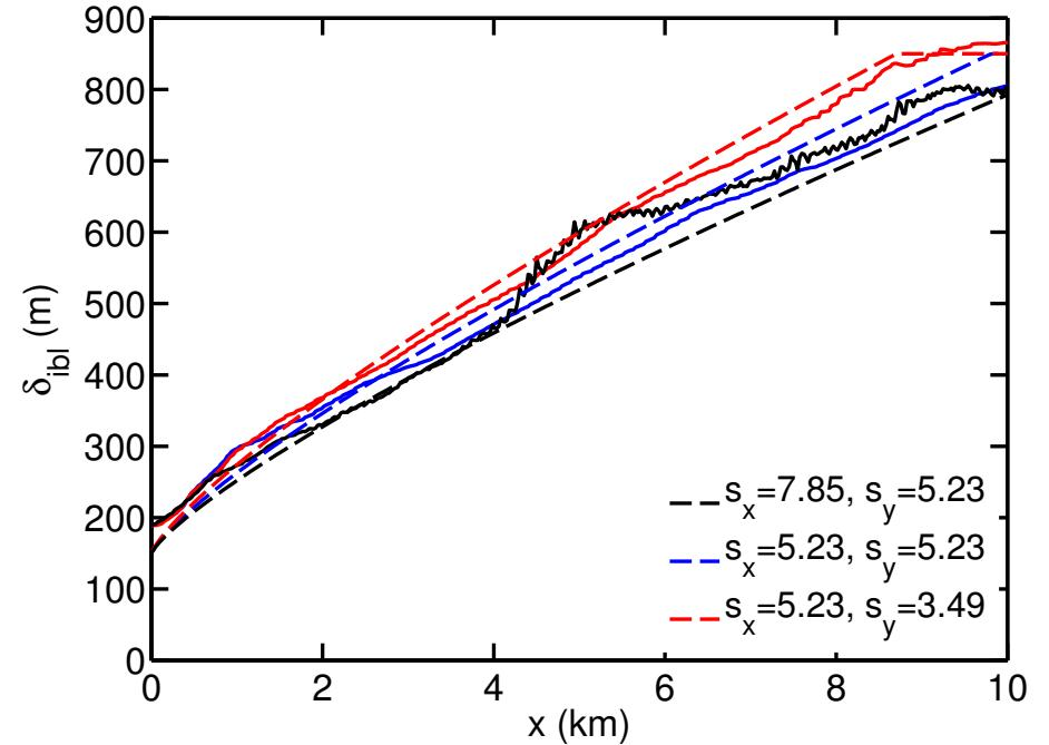
Internal boundary layer finite size wind-farm
