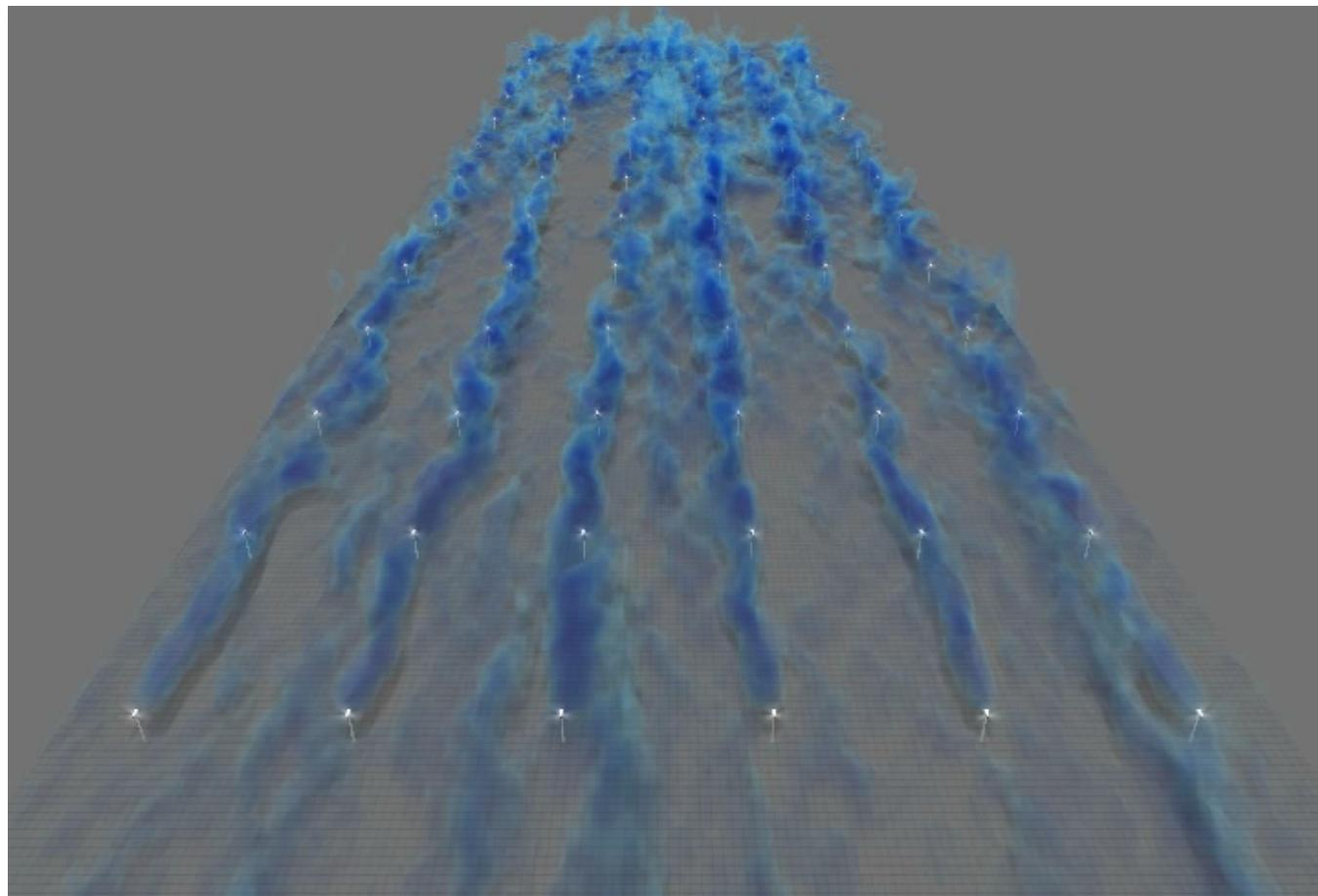
In-silico wind farm (Large-Eddy-Simulation) JHU-LES code
