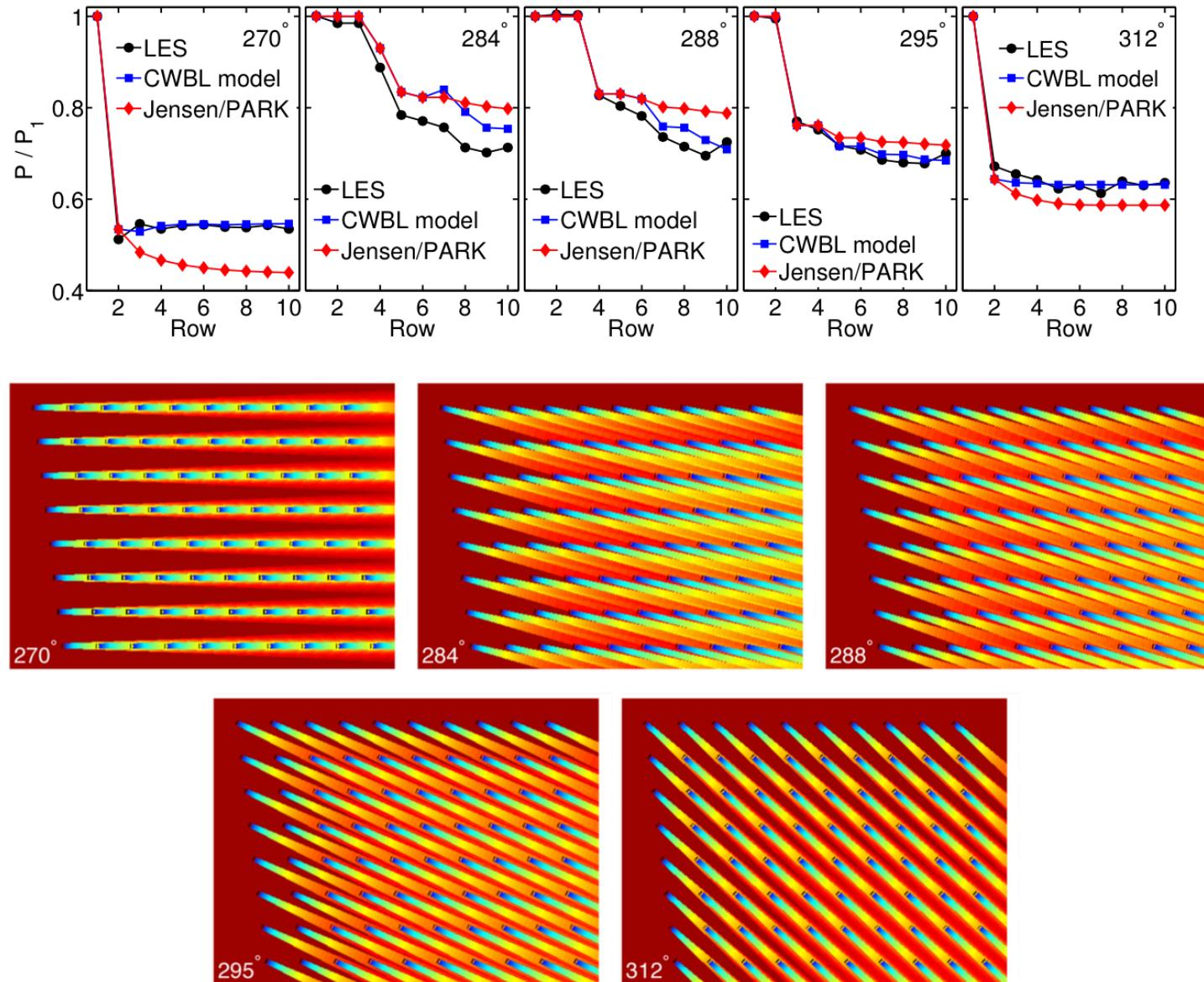
**Figure 6.** Comparison between the LES results from Porté-Agel [2] (black circles), the CWBL model (blue squares) and the Jensen/PARK model (red diamonds) for Horns Rev. The top panels indicate the results for the wind-directions  $270^\circ$ ,  $284^\circ$ ,  $288^\circ$ ,  $295^\circ$ , and  $312^\circ$ . The lower panels show a visualization of the normalized velocity field at hub-height obtained from the CWBL model for these cases.
