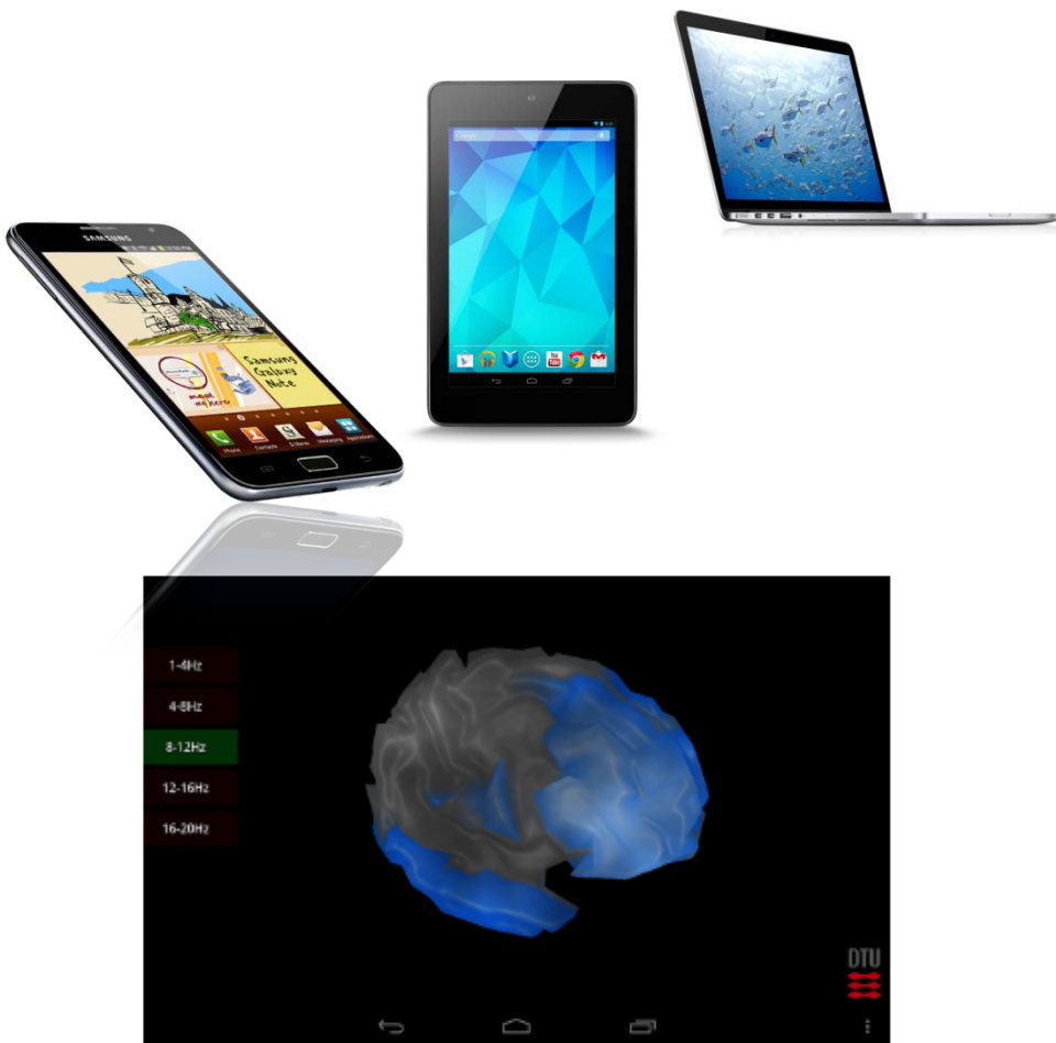
Fig. 5: The 3D brain visualization application running on a Nexus 7 tablet. Blue color indicates cortical activity in the 8-12 Hz band.
