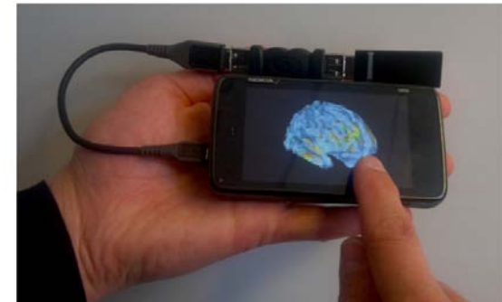
Fig. 3. A user interacting with a 3D model of the brain using the handheld brain scanner device with touch-based interaction.
