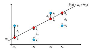
**Example**: Fit data with linear function  $\hat{y}(\mathbf{x}) = w_1 + w_2 \mathbf{x}$  by finding the parameters  $\mathbf{w} = (w_1, w_2)$ .
