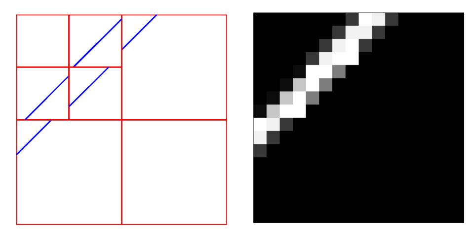
80 bits to jointly encode 5 wedgelets
