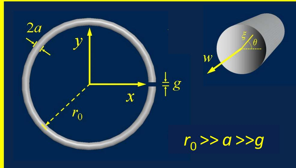
$$Z_{\text{spr}} = i \left( \frac{4\pi r_0 \omega}{ka\epsilon_S^{-1/2} c^2} \right) \frac{J_0(ka\epsilon_S^{-1/2})}{J_1(ka\epsilon_S^{-1/2})} - i \left( \omega L / c^2 - 1 / \omega C \right)$$
