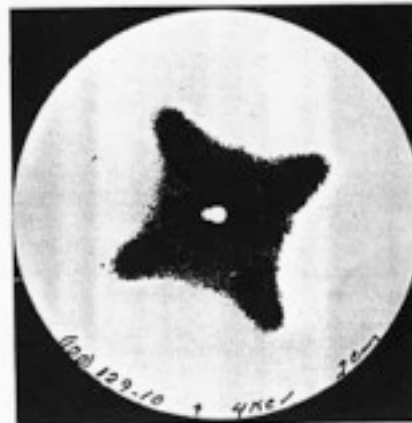
FIGURE 17. An experimental dN/dE distribution (spot pattern) for Cu(001)-Ar + (001)-4.0 keV captured on a plane glass plate. The ion beam entered through the central (white) hole. (From Sushers, A. L., Willis, W. R., and Robinson, M. T., J. Appl. Phys. , 34, 153, 1963. With permission.)
