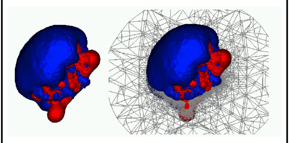
Potential contours from solution to linear PBE for FAS2 shown with a slice through the finite element mesh. Solution was computed using the adaptive finite element software MC.
