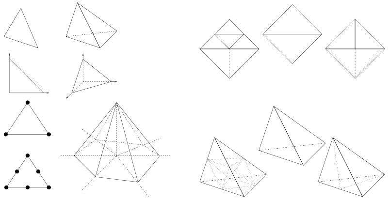
Error-estimate-driven adaptive finite element methods often based on simplex subdivision. (Above: 2/4/8-section and conformity.)
