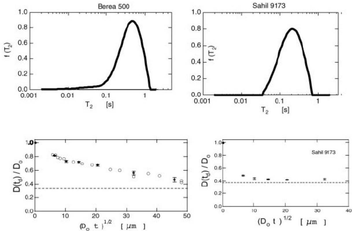
**Figure 13** Relaxation time distribution in two very dissimilar rocks—Berea permeability about 0.17 Darcy (1 Darcy = 1  $\mu\text{m}^2$ ) with relatively uniform pores and a carbonate with coexistent macro- and micro-porosity, with a permeability about 16 times smaller. The distributions are rather similar and the pore-size distribution from relaxation data alone cannot be made. Time-dependent diffusion coefficient reveals clearly the differences between these two dissimilar rocks.
