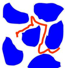
Carbonate: Similar  $T_2$  Distribution, Different Pore Geometry
