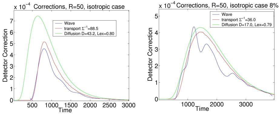
Correction generated by an inclusion of radius R=50 where the random fluctuations are suppressed. Left: 5% RMS. Right: 8% RMS. Transport and diffusion generated by best energy fit. The diffusion fit is now much more accurate.
