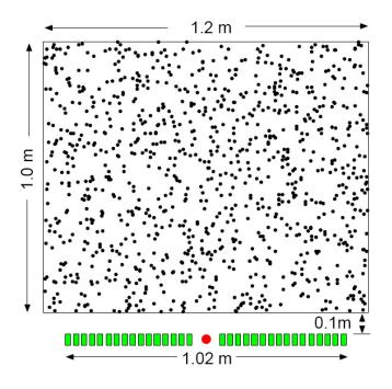
All subsequent reconstructions based on frequency average on the interval [9GHz, 11GHz]. Best fit for mean free path is 42cm (91cm for band [6.5GHz, 8.5GHz], showing behavior of mfp in  $k^{-3}$ ).
