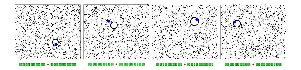
Reconstruction of four holes created by the removal of three rods. Reconstruction based on differential measurements.
