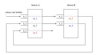
If the red buffers have higher priority than the blue buffers, jobs in buffer 2 and buffer 5 can *never* be processed simultaneously. Mathematically,
