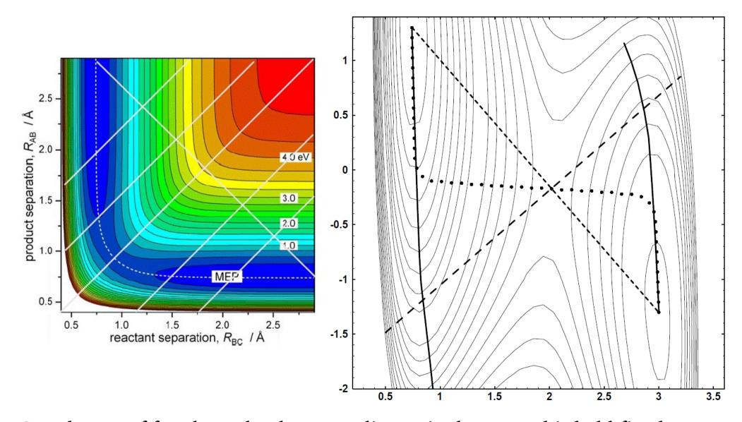
One degree of freedom, the drag coordinate, is chosen and is held fixed while all other D-1 degrees of freedom are relaxed, i.e. the energy of the system minimized in a D-1 dimensional hyperplane.
