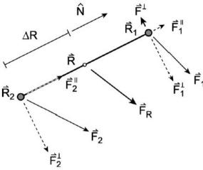
The dimer is rotated in order to find the lowest curvature mode of the potential energy at the point where the dimer is located.
