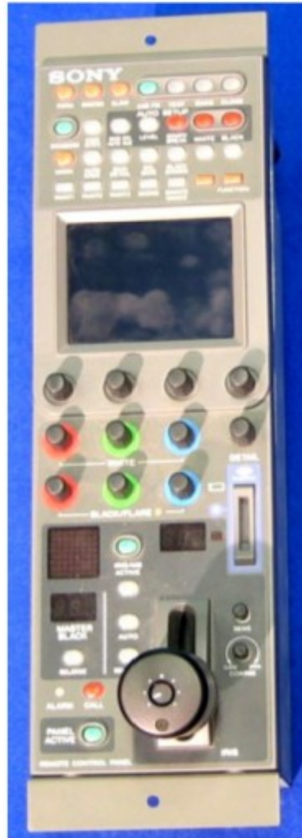
Figure 2.5: A close-up of a camera control unit (left), and Four camera control units as used by a “racks operator” in an outside broadcast truck (right)
