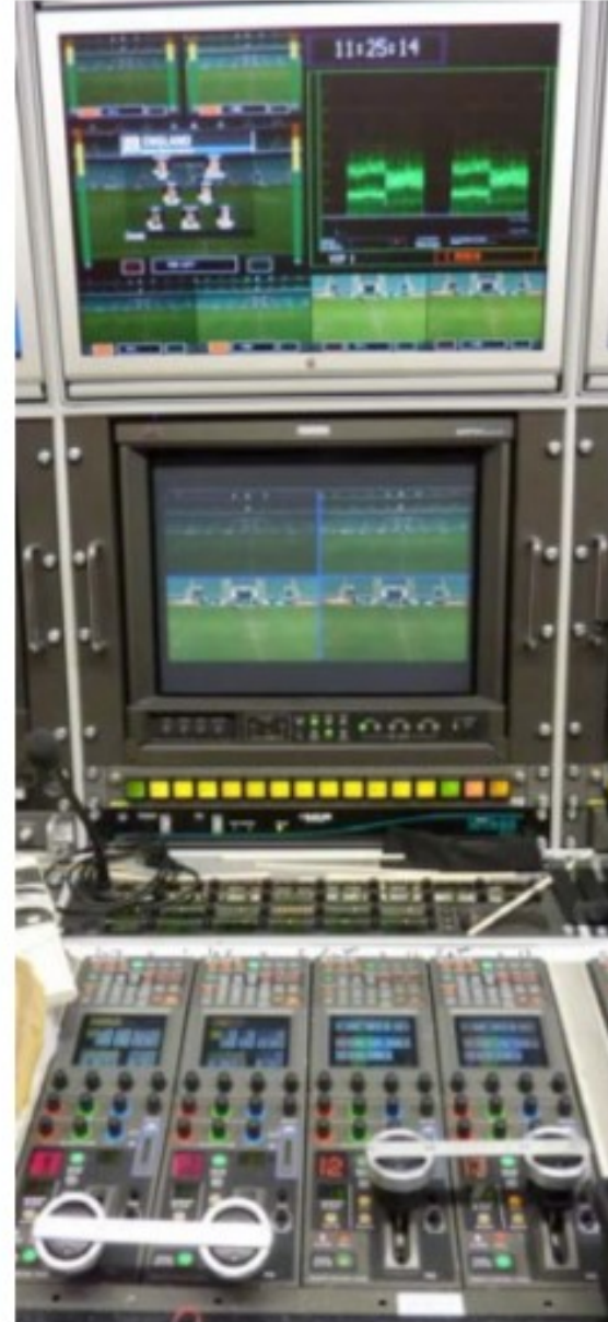
Figure 2.5: A close-up of a camera control unit (left), and Four camera control units as used by a “racks operator” in an outside broadcast truck (right)
