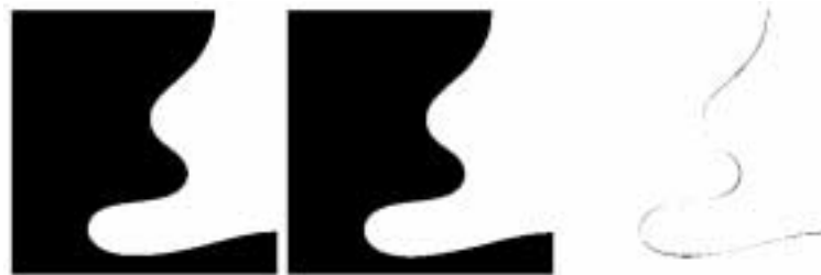
Figure 18.2: Comparison of the iterated median filter and of the curvature motion. Numerically, the iterated median filter and the curvature motion are very close, when the curvatures of the level lines are not too small. Indeed, the iterated median filter converges towards the viscosity solution of the curvature motion. Left : simple shape smoothed by a finite difference scheme of the curvature motion, middle : smoothing by a median filter a the same scale, right : difference between left and middle images. The difference is not larger that one pixel width.
