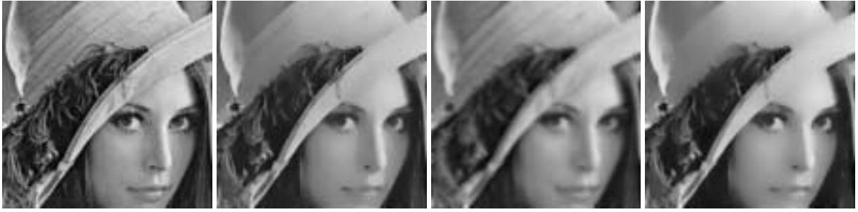
Figure 1.12: A proliferation of diffusion models. From left to right: Original image, Perona and Malik equation 1987, Zhong, Carmona 1998 (diffusion along the least eigenvector of D^2u ) and Sochen, Kimmel and Malladi, 1998 (minimization of the image graph area).
