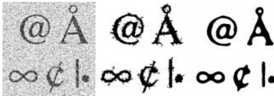
Figure 24.11: Finite difference scheme for AMSS. Left : Original noisy image of letters, middle : same image without the extrema with area less than 80 pixels (extrema killer). Right : result of AMSS at calibrated scale 4.
