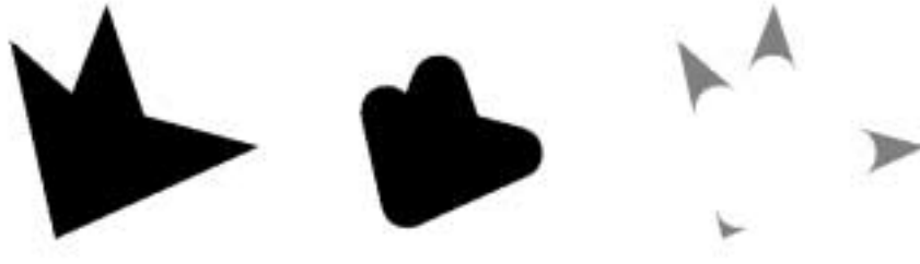
Figure 9.4: Opening of a set as curvature threshold from above. A set X , its opening by a ball of radius 20, and the difference between original and processed. This opening transforms X into the union of all balls of radius 20 contained in it. The resulting operation can be understood as a threshold from above of the curvature of the set boundary.
