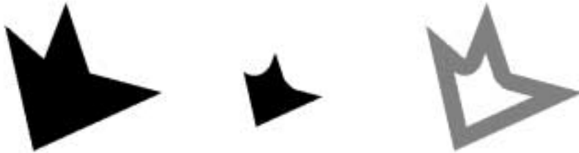
Figure 9.2: Erosion of a set. A set X (in black), its erosion by a ball of radius 20, and the difference set.
