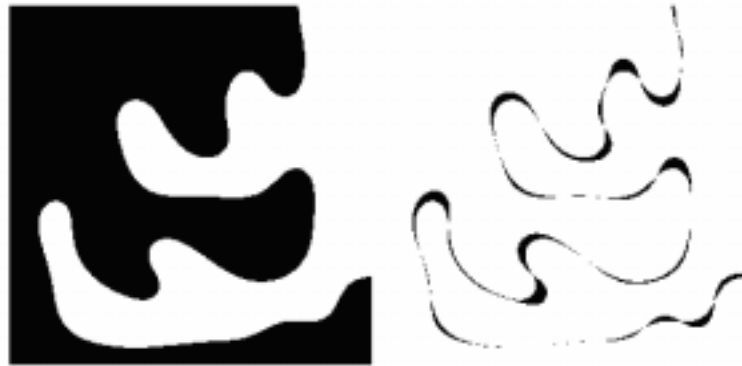
Figure 11.2: Median filter and the curvature of level lines. The median filter does a smoothing linked to the curvature of the level lines. Left : image of a simple shape. Right : difference of this image with itself after it has been smoothed by one iteration of the median filter. We see, in black, the points which have changed. The width of the difference is proportional to the curvature, according to Theorem 11.3.
