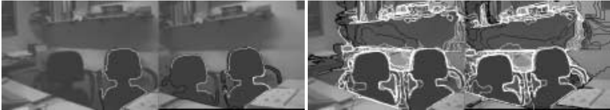
Figure 1.23: Level lines based shape parser. Shape extraction has ever been the bottleneck of shape recognition algorithms. With the presented algorithm, this problem is solved by a brute force method : it compares all level lines of the images to be compared. Left pair of images : two images of a desk taken from different angles. In the left hand desk image, one level line has been put in white. We display, also in white, in the right image of the pair, the matching level lines. The match is ambiguous, as must be expected when the same object is repeated twice in the scene ! In the right pair of images, we display in white all matching pairs of level lines. (Experiment : J.-L. Lisani).
