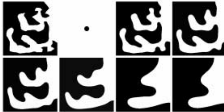
Figure 18.1: Scale-space based on iterations of the median filter. From left to right and up to down : original shape, the size of the disk used for the median, and the result of the iterated median filter for an increasing number of iterations.
