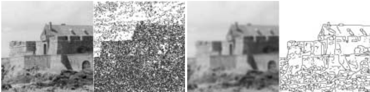
Figure 1.10: Heat equation and Canny’s edge detector. Boundaries, or “edges” of the image can be defined as points where the gradient attains a maximal and large value along the gradient lines. This amounts to say that edge points are points where D^2u(Du, Du) crosses zero and |Du| is large. Canny’s edge detector computes those points. On the left, the original image, followed by the edge points found. They make a very dense set, because of the oscillatory character of the image. Next, the image blurred by the Gauss kernel (heat equation) and the Canny edges found. The heat equation has removed the “irrelevant” edges (Chapter 3)
