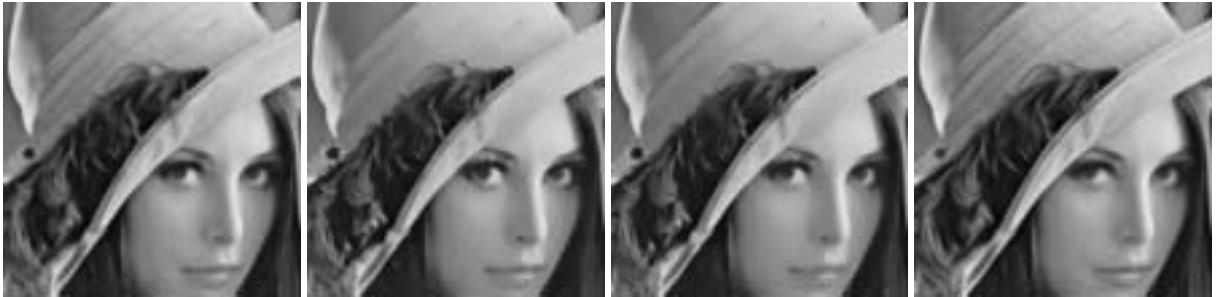
Figure 1.14: A proliferation of diffusion models (II). From left to right: Osher, Sethian 1988: curvature equation, Rudin, Osher and Fatemi 1992: minimization of the image total variation, Alvarez, Lions et al. : nonlocal variant of the preceding, 1992, Weickert 1994 : nonlocal variant of the curvature equation. All of these models only diffuse in the direction orthogonal to the gradient, with a more or less local estimate of this direction.
