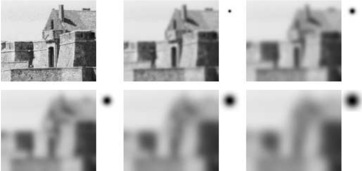
Figure 2.4: Convolution by gaussian kernels (heat equation). From top-left to bottom-right, we display the original image, and the results of the convolutions with gaussians of increasing variance. A grey level representation of the convolution kernel is put on the right of each convolved image ; it gives an idea of the size of the involved neighborhood. The resulting image is more and more blurry.
