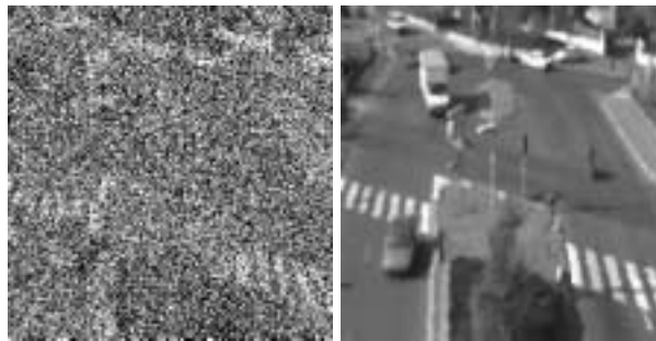
Figure 1.2: Denoising. A second goal of image processing : the restoration. Left: original noisy image (simulated salt and pepper noise up to 75%), right: denoised version
