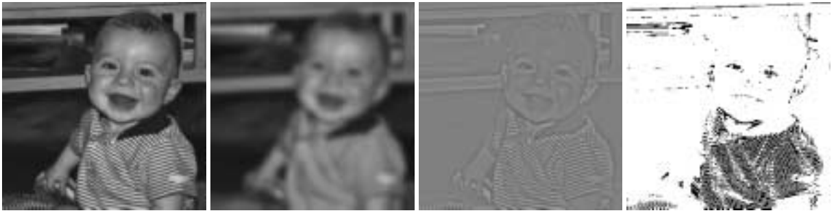
Figure 1.9: The “laplacian pyramid” of Burt and Adelson. From left to right : original image, image blurred by gaussian convolution, then difference between the original image and the blurred version, which simulates the laplacian of the original image. In black in the last image, points where this laplacian image is large. This experiment simulates the first step of the laplacian pyramid. The laplacian image is, for most digital images, a sparse representation, therefore well adapted to compression.
