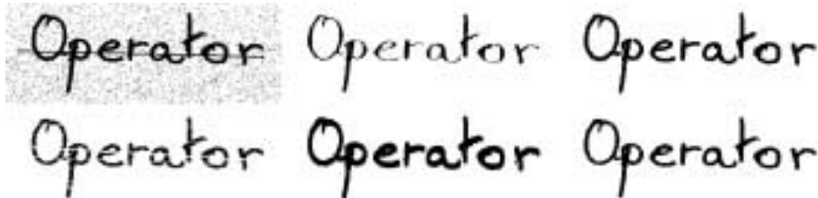
Figure 9.8: Opening and closing based denoising. On the first row : scanned picture of the word “operator” with black dots and a black line added, a dilation with a 2 \times 5 rectangle (middle), then an erosion with the same structuring element. The resulting operator is a closing. Small black structures are removed by a such process. In the second row : the word “operator” with a white line and white dots inside the letters, erosion with a rectangle 2 \times 5 , followed by a dilation. The resulting operator is an opening. Small white structures are removed.
