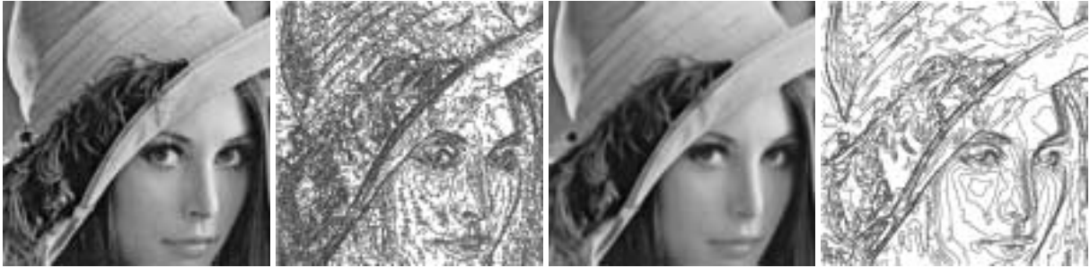
Figure 1.18: The Affine and Morphological Scale Space (AMSS model). From left to right : original image, level lines of the images (16 levels only), smoothed image by using the affine and morphological scale space, and its level lines (Chapter 6).
