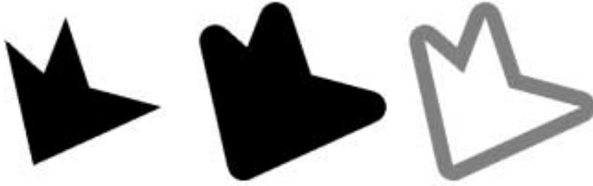
Figure 9.1: Dilation of a set. A set X (in black), its dilation by a ball of radius 20, and the difference set.
