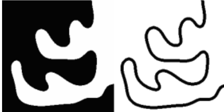
Figure 11.1: The erosion does a smoothing independent of the curvature of the level lines. Left : image of a simple shape. Right : difference of this image with its eroded by a ball with radius 6. We see in black the points which have changed. The width of the difference is constant.
