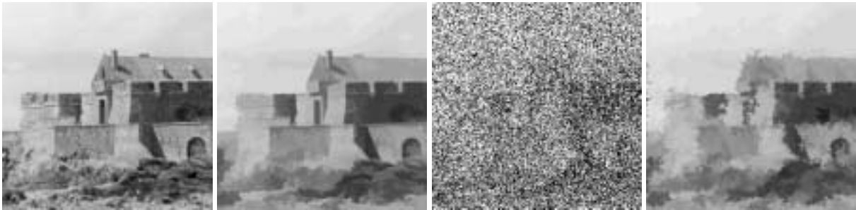
Figure 1.16: The "extrema killer" filter : all connected components of the upper or lower level sets with small area are removed from the image. From left to right : original image, extrema killer applied with area 80 pixels, then 75% salt and pepper noise added to the original image and the same filter applied (Chapter 7).
