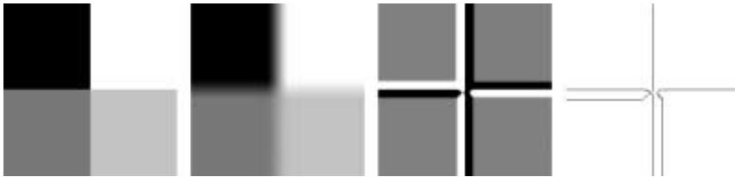
Figure 3.5: Zero crossings of the Laplacian of a synthetic image. From left to right : the original image, the image linearly smoothed by a convolution with a Gauss function, the sign of the Laplacian of the filtered image (the gray color corresponds to values close to 0, black to clearcut negative values, white to clearcut positive values) and the zero-crossings of the Laplacian. This experiment clearly shows the drawbacks of the Laplacian as edge detector.
