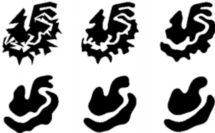
Figure 3.12: The Bence-Merriman-Osher shape smoothing method is a localized and iterated version of the Dynamic Shape method. A convolution of the binary image with small-sized gaussians is alternated with mid-level thresholding. It uses (top, left) as initial data the same shapes as in Figure 3.4. From top to bottom and left to right: smoothing with increasing scales. Notice that the shapes keep separate. In fact, there is no interaction between their evolutions. Each one evolves as it would do alone.
