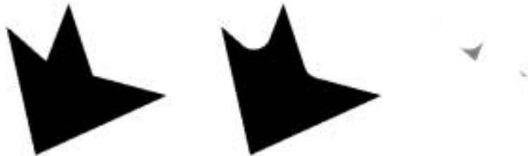
Figure 9.5: Closing of a set as a curvature threshold, from below. A set X , its closing by a ball of radius 20, and the difference between original and processed. The closing of X is nothing but the opening of X^c . It can be viewed as a threshold from below of the curvature of the set boundary.
