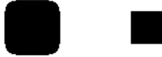
Figure 17.2: Erosion and dilation can generate singularities within the level-lines. Left : original image where the only level-line, corresponding to the boundary of the black shape, is C^2 . Right : erosion with a circle of radius 10 : the resulting level-lines have angles.
