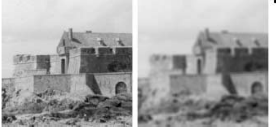
Figure 2.1: Local averaging algorithm. Left : original image, right : result of replacing the grey level at each pixel by the average grey level over the neighboring pixels. The shape of the neighborhood is defined by the black spot displayed up-right.
