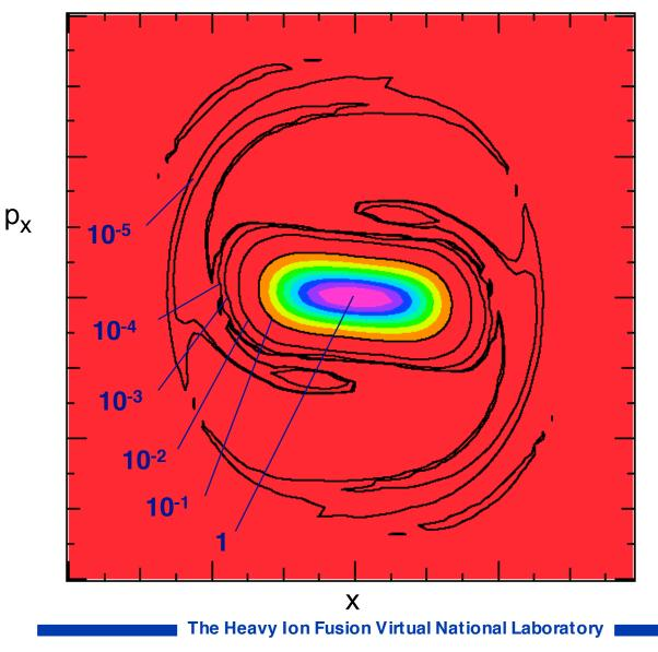
4D Vlasov testbed (with constant focusing) showed structure of the halo in a densitymismatched beam
