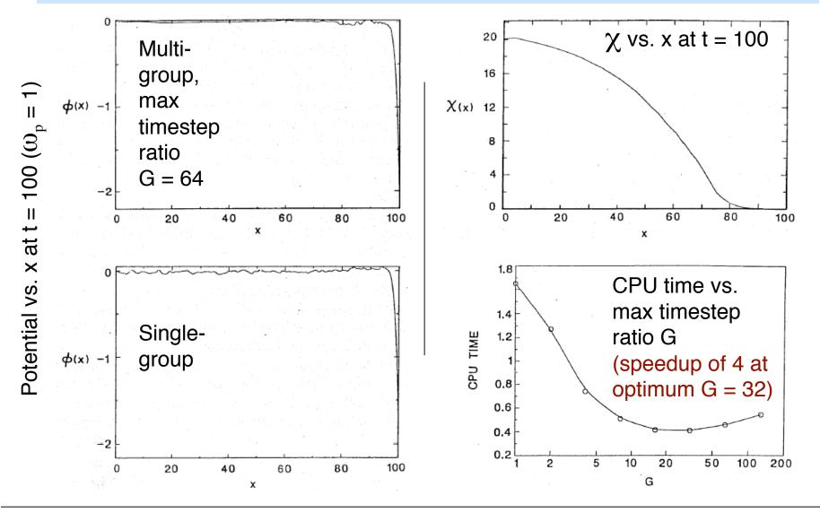
Another series of runs examined propagation of an ion acoustic shock front toward a conducting absorbing plate; see paper by Parker, *et al.*
