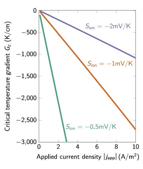
Dendrite suppression by thermal gradients is most effective during slow charging and least effective during fast charging, consistent with experiments
