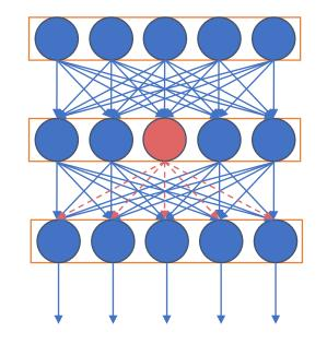
Since the output of the neuron is always zero, we can easily remove it from the neural network
