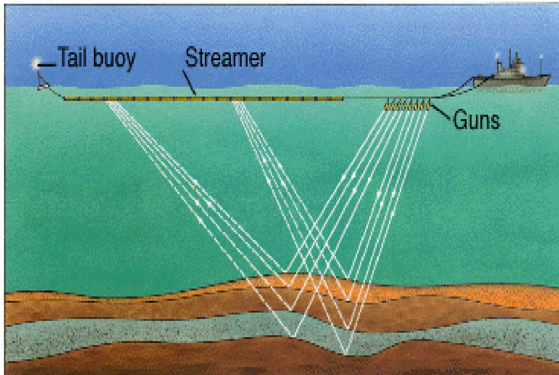
Typical distances: streamer length = 3 - 8 km, source spacing  $\simeq$  hydrophone spacing = 10 - 25 m, parallel *sail lines* spaced 25 - 150 m apart.
