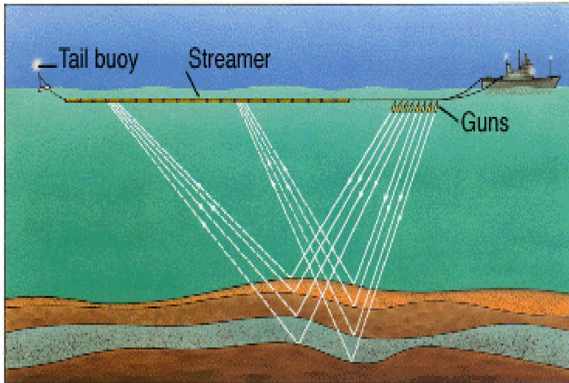
Ship tows *source* (compressed air gun) and *receivers* (hydrophone streamer). Typically records 100's of channels - recently 1000's. [thanks: Schlumberger]
