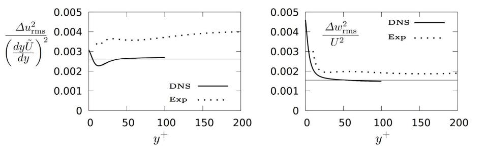
The DNS data are for a plane channel with  $Re_{\tau} = 2000$  and 5200 (Lee & Moser (2015)) The experimental data are for a zero pressure gradient boundary layer with  $Re_{\tau} = 3000$  and 10500 (Baidya *et al.* 2012)
