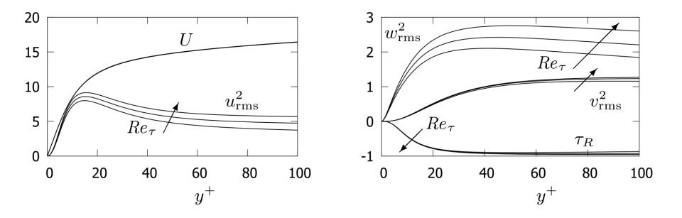
DNS data for  $Re_{\tau} = 950$ , 2000 and 5200 showing that  $u_{\rm rms}^2$  and  $w_{\rm rms}^2$  vary with  $Re_{\tau}$  significantly more than  $U, v_{\rm rms}^2$  and  $\tau_R = \langle u'v' \rangle$ .
