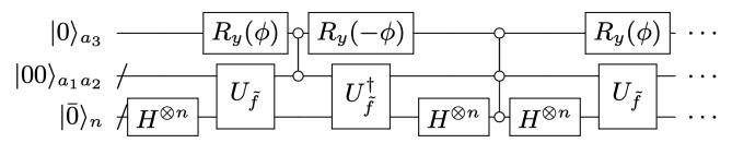
3. Amplitude amplification (exact) circuit
