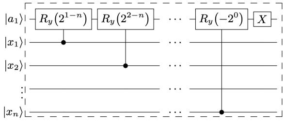
1.  $U_{\sin}$  block encoding circuit
