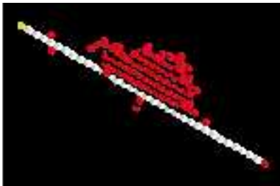
Figure 6: Chain Behavior. The Proteo system is shown here half-way to a complete chain. The colors indicate the current module states: white modules have settled (FINAL mode) and red modules are still looking for a place in the structure (SEARCH mode). The yellow module is the current SEED.
