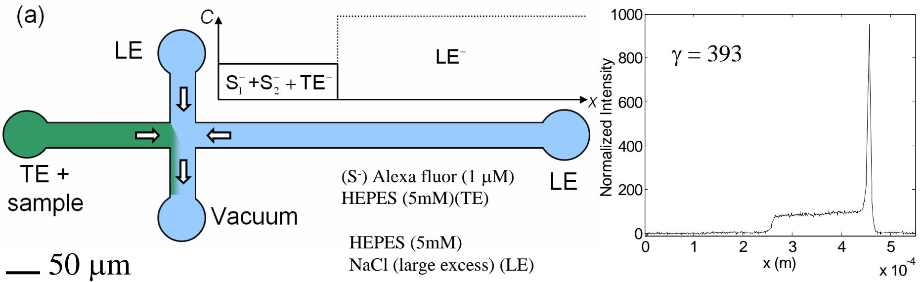
Demonstrated  $>1\text{e}6$ -fold stacking on chip
