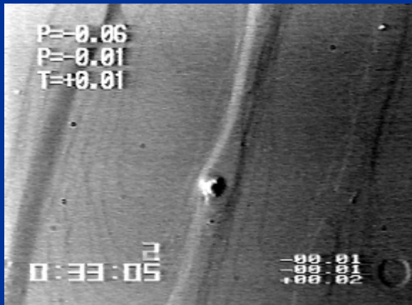
Dried lipid film on glass cover slip showing lamellar structure
