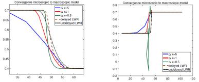
• Two special scenarios: rarefaction wave (left) and shock wave (right)
