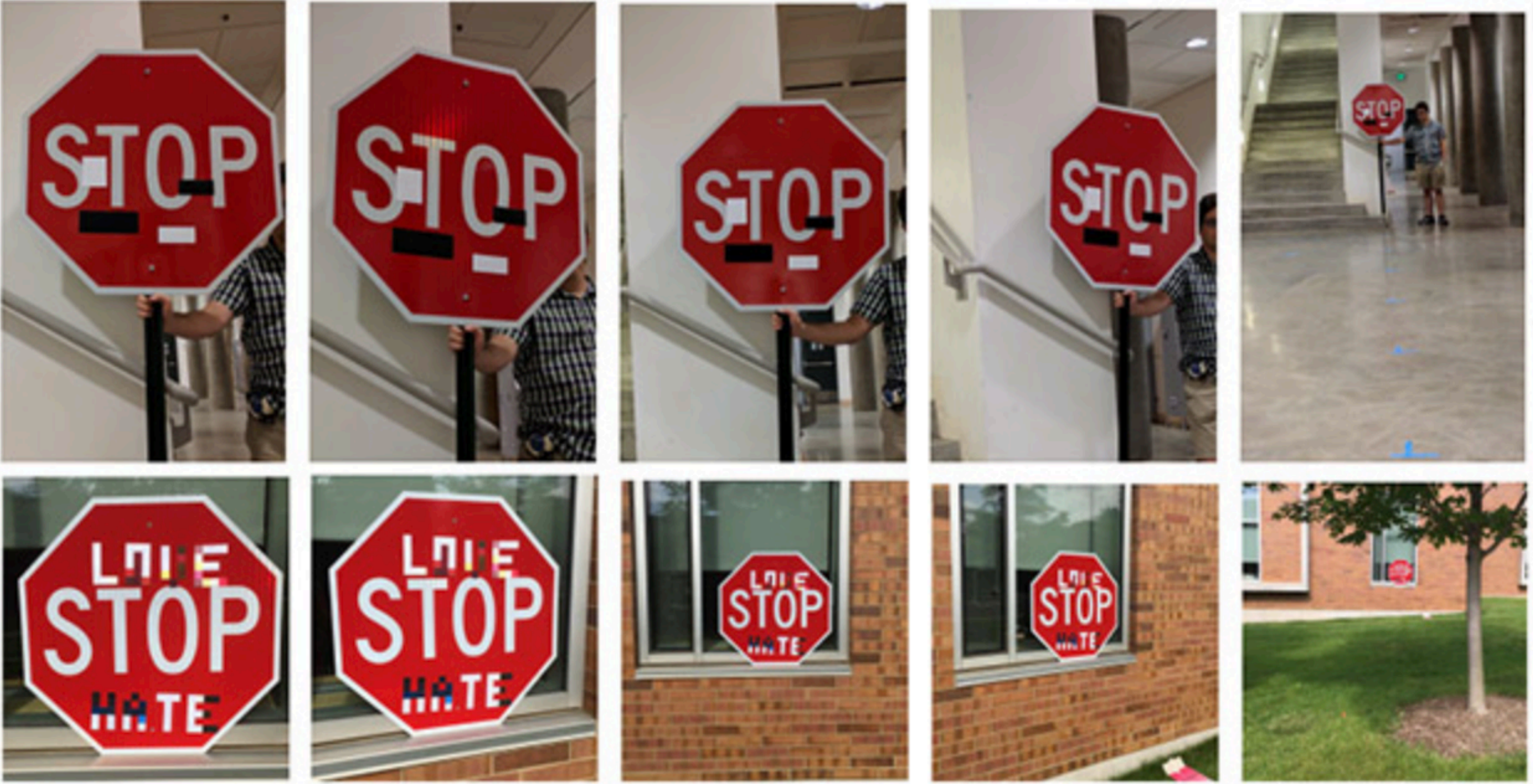
Images: Evtimov et al Camouflage graffiti and art stickers cause a neural network to misclassify stop signs as speed limit 45 signs or yield signs.
