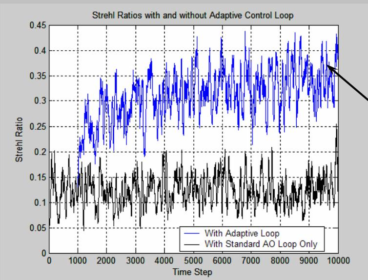
**Adaptive control loop significantly improves beam control and increases intensity of energy focused on target.**
