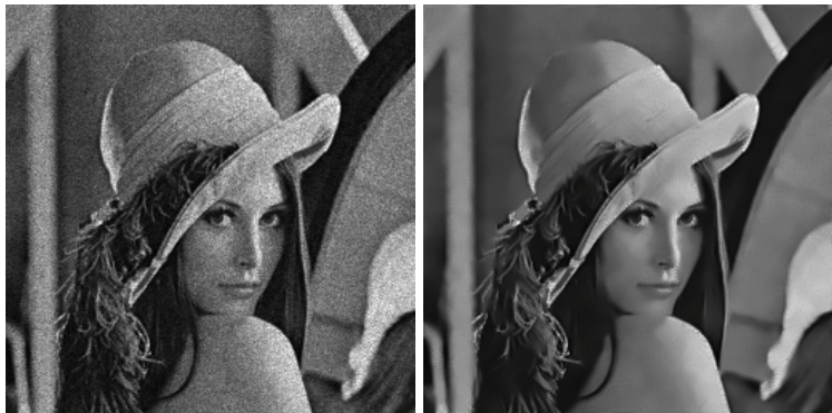
Figure: Poisson corrupted image (left) denoised using the patch graph (right).
