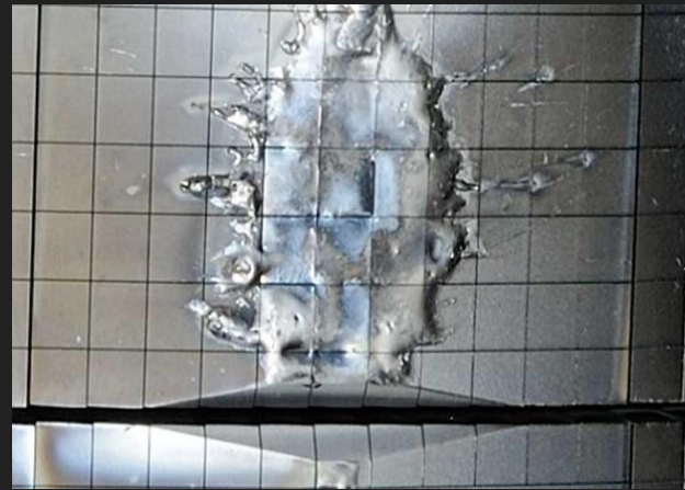
JET runaway electrons damage. https://www.iter.org/newsline/-/2234
