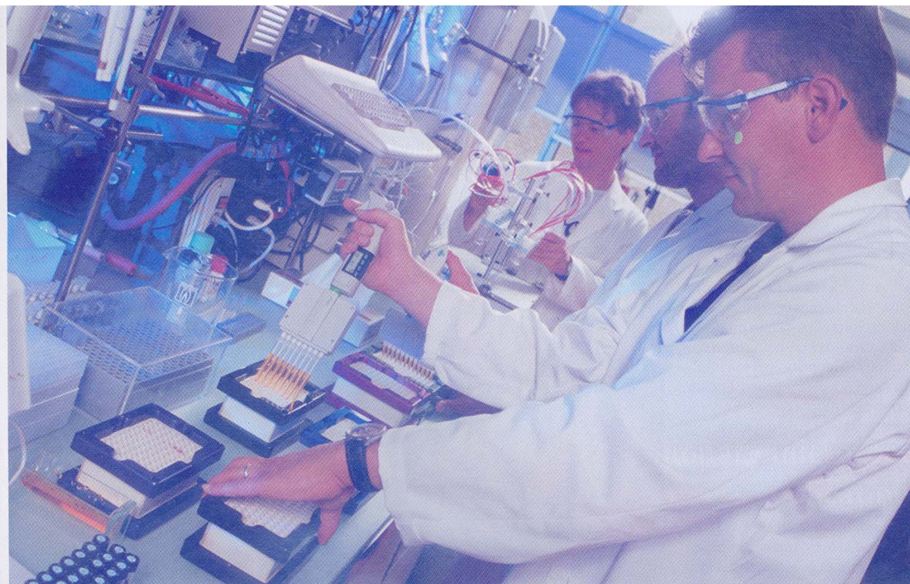
MANY AT A TIME Program head Andreas Marzinik (front to back) and lab specialists Raphael Gattlen and Urs Rindisbacher of Novartis Pharma AG, Basel, Switzerland, pipette coupling reagent into 96-well reaction blocks.
